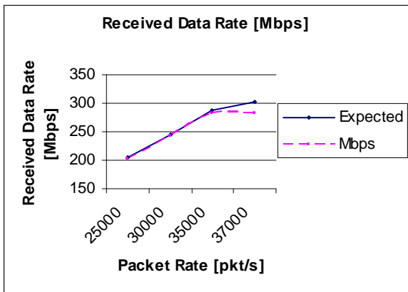
Figure 31: Received data rate over Windows platform (distributed and log at receiver side)
